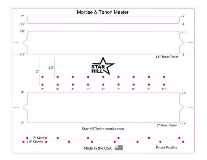
**General Use Instruction**: For each layout function, determine and mark the starts and stops for the joinery. Then, align the reference edge, snap line, or center line to the Mortise & Tenon Master (long edge or V-groove); mark your start and stop lines perpendicular to the timber.
