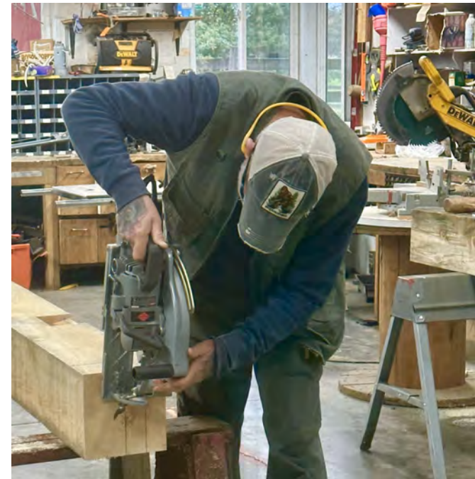
Drop cutting a tenon
