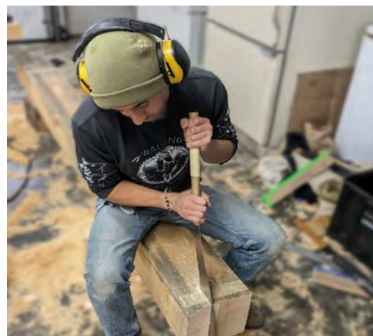
Cutting a tenon by hand, using a Japanese Boat Saw
