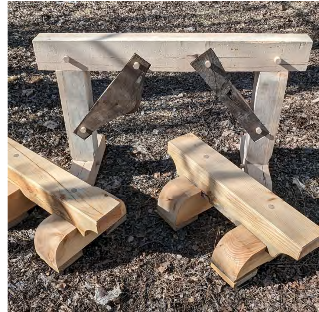
Sawhorse with "Let In" braces, the small set of horses is used for chain mortising and drilling
