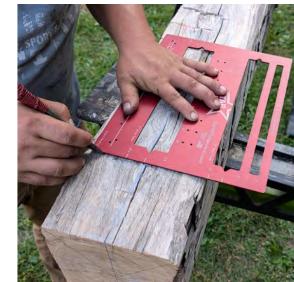
The Mortise and Tenon Master works very well for centerline layout, used for ridges to accept rafters
